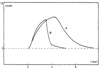
Figure 6. Fractograms of a 66.5 SAN/23.5 Solprene 411/10 copo PB-PMMA blend (curve A) and of ABS Cycolac GSM (curve B). Charpy impact tests on notched specimens DIN 53453.
